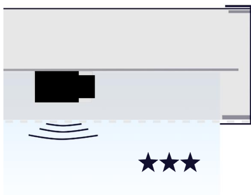
Figure 3: In case of a metal fixture place the micro BLC 0-10V industrial on the side of the light diffuser.
