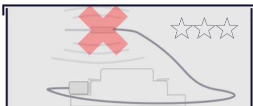
Figure 9: Do not place the antenna in a metal housing / junction box.
