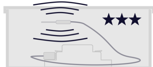
Figure 10: Freely place the antenna in a plastic junction box / housing (not against plastic)
